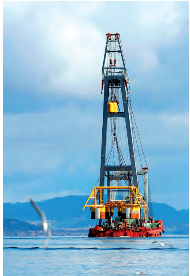
The self-propelled heavy lift crane vessel UGLEN, with a lifting capacity of 600 tonnes. Photo: Geir Otto Johansen, Statoil
